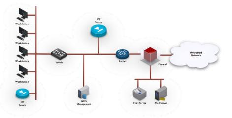
Figure 1: A typical network topology of a NIDS.
