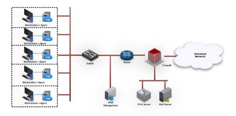
Figure 2: A typical network topology of a HIDS.
