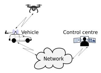
Figure 5: Option of using a fixed network for transmission of sensor data.
