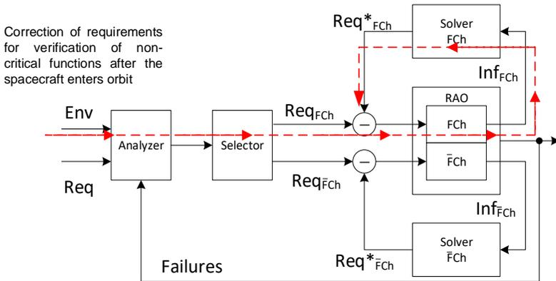
**Figure 4: Scenario 1. Online re-verification of non-critical functions.**
