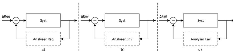
**Figure 1: Circuit models of the resilience management system: when changing the requirements for the system (a), when changing the parameters of the environment (b), when changing the failures of the system (c).**
