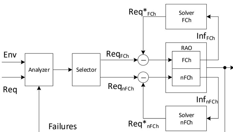
**Figure 2: Integrated cybersecurity control system of the information system structure:** FCh – Functional Characteristic, nFCh – non - Functional Characteristic, RAO – Resilience assurance object.
