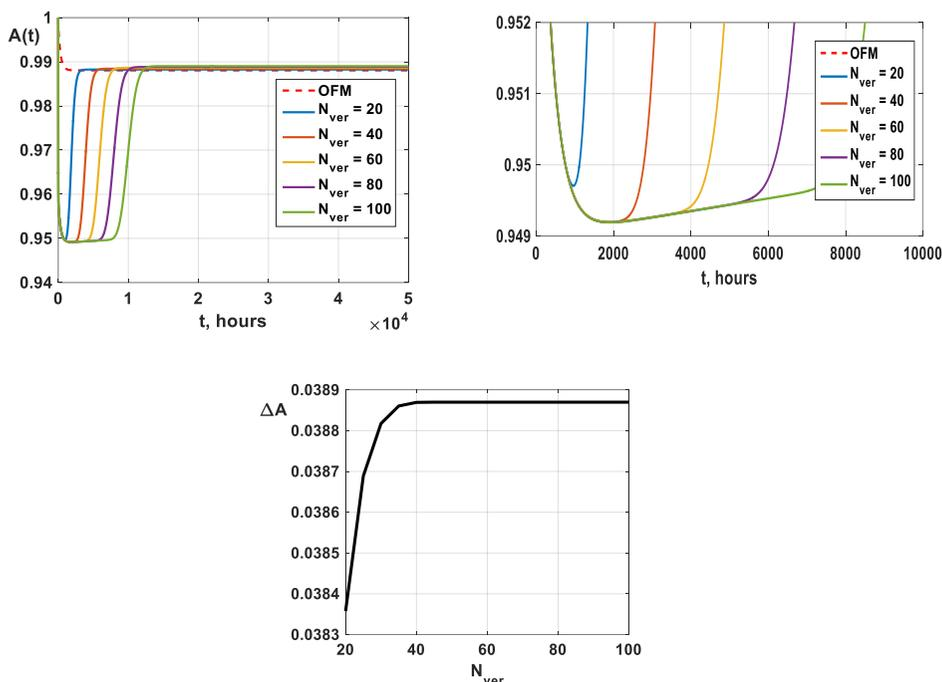
**Figure 7: The results of modelling the COV according to the scenario 1 (verification of non-critical functions after start of the spacecraft).**
