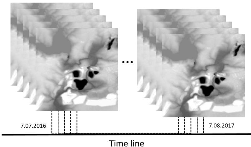
**Figure 3: Terrain elevations maps time series from radar interferometry.**
